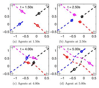
Fig. 7. Trajectories of 4 robot agents with decentralized swarm barrier certificate. The arrow, circle and dashed line represent current velocity, current position and trajectory the agent.  $D_s = 0.2m, \gamma = 0.1$
