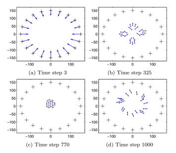
Fig. 2. Simulation of centralized swarm barrier certificate with 20 mobile robot agents, the arrow represents current velocity of the agent,  $D_s = 10$
