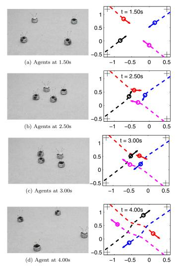
Fig. 6. 4 robots with centralized swarm barrier certificates. The arrow, circle and dashed line represent current velocity, current position and trajectory of the agent,  $D_s = 0.2m, \gamma = 0.1$ . Units for X and Y coordinates are in meters. A video can be found Online (2015).
