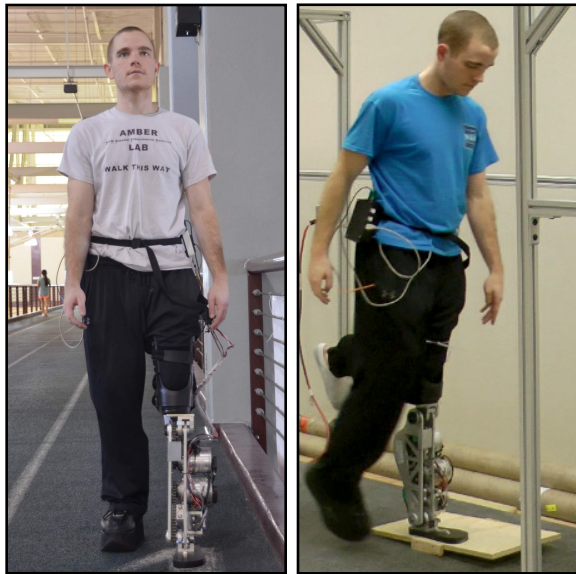
Figure 1: The novel Prosthesis AMPRO that is capable of running nonlinear optimization based controllers in real-time.
