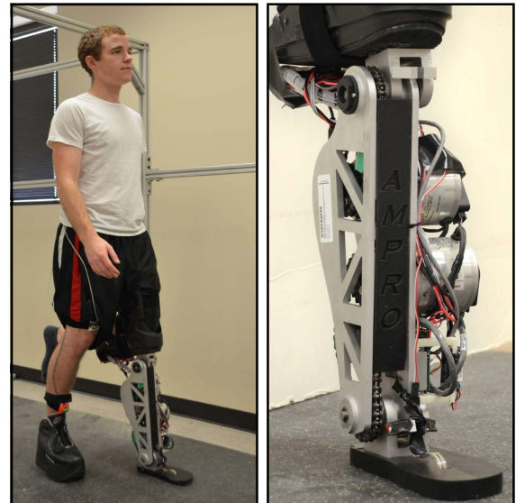
Figure 1: Transfemoral prosthetic: AMPRO.
