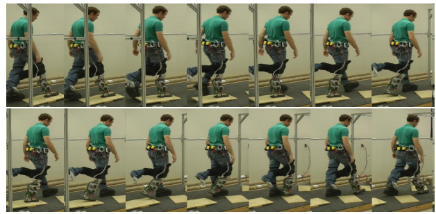
Figure 3: Gait tiles of walking over obstacle.
