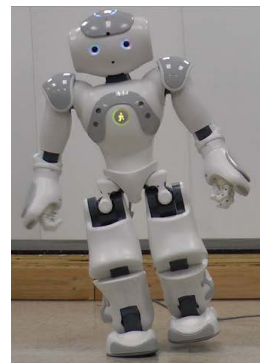
Figure 1: Experimental demonstration of NAO displaying dynamically stable walking.
