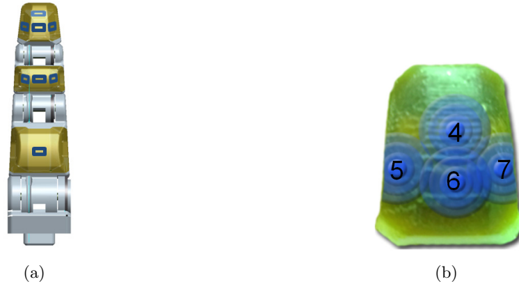
Figure 3: (a)The barometers in each finger (dark rectangles). (b)The distal barometer spatial sensitivity.
