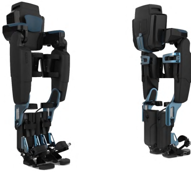
FIGURE 1. Image of Exoskeleton from Wandercraft. Link names with respective mass values are presented in Table 1.
