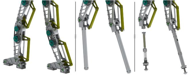
Fig. 4: Model views of the leg configurations tested on AMBER3M in the presented experiments: Flat Foot (left), Point Foot (center), Compliant Point Foot (Right).
