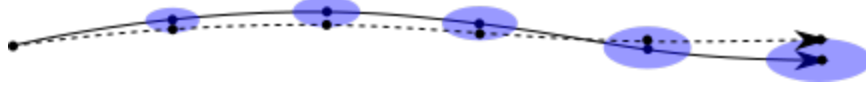
Figure 1: Example base trajectory and uncertainty region, where the solid trajectory is a base trajectory \mathbf{x}_i \in \mathcal{B} , and the dashed line is a trajectory in \Omega , the blue ellipses are the uncertainty region determined by the atom set \mathcal{A} .
