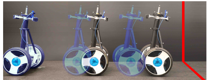
Fig. 1. Visualization of desired Segway behavior. The Segway is driven from left to right and must not cross the red line. The transparent blue images represent the measured position whereas the opaque images represent the true position. Traditional CBFs do not account for this uncertainty.
