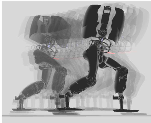
Fig. 1: The humanoid robot, DURUS, running stably in 3D in a simulation environment as a result of a large-scale hybrid zero dynamics optimization. This study presents the result of 25 gait optimizations achieving a range of running speeds.
