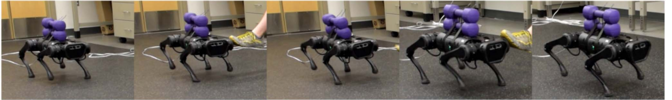
Fig. 2. This experiment displays A1 trotting under the influence of both a 4.54 (kg) payload (36% of the robot's weight) and push disturbances. The quadruped was able to resist these uncertainties and continue trotting. Videos of the experiments are available online [28].
