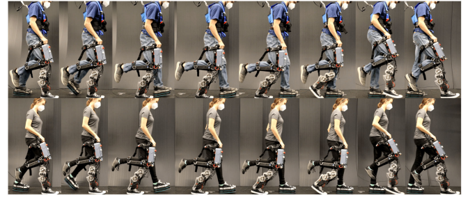
Fig. 4. Gait tiles of 2 subjects walking on a rubber floor with the force sensing ID-CLF-QP prosthesis controller.
