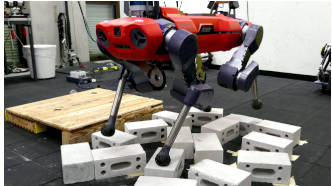
Fig. 1. ANYmal [6] performing a trotting gait on stepping-stones.
