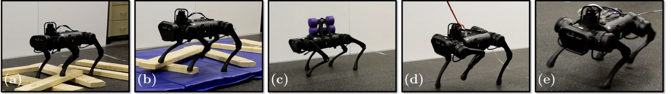
Fig. 1. Snapshots illustrating the performance of the distributed QP-based controllers for a series of blind locomotion experiments (indoor) on the quadrupedal platform, A1. (a) Forward locomotion in a field of arbitrarily dispersed wooden blocks at 0.5 (m/s), (b) trotting on a compliant surface (gym mat) scattered with wooden blocks at 0.4 (m/s), (c) forward locomotion with a payload of 4.54 (kg) (%36 uncertainty) at 0.5 (m/s), (d) tethered pulling while trotting in-place, and (e) stabilization in the presence of external disturbances. Videos of all experiments are available online [36].
