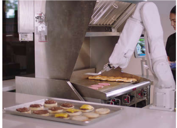
Fig. 1: Figure showing a typical burger cooking apparatus. The grill is where the burger is cooked, and the table is where the freshly cooked burger is placed. We are using this setup for deploying the techniques described in the paper as it cooks burgers in real-world restaurants. A video demonstration is shown in this footnote 1 .
