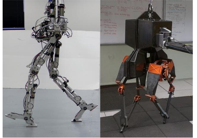
Fig. 4: Bipedal robots AMBER2 (left) and ATRIAS (right).
