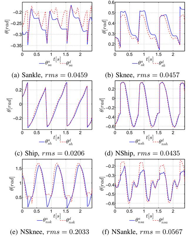
Fig. 14: Actual vs. desired joint angles logged during AMBER2 walking with the unified control law, with  $rms$  the root mean square of tracking error.
