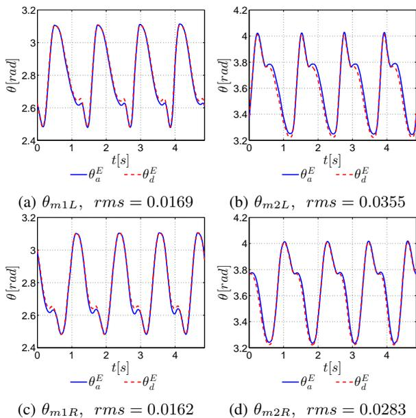
Fig. 16: Comparison of the actual  $\theta_a^E$  versus desired  $\theta_d^E$  motor angle trajectories of left leg ( $\theta_{m1L}, \theta_{m2L}$ ) and right leg ( $\theta_{m1R}, \theta_{m2R}$ ) from experiment.
