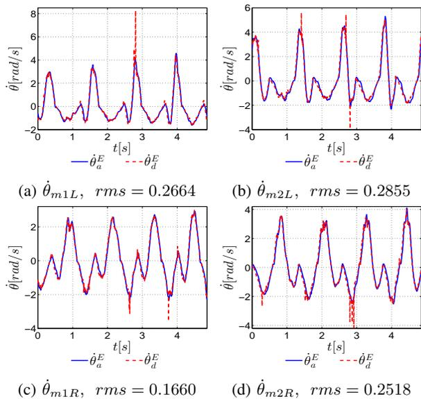
Fig. 17: Comparison of actual  $\dot{\theta}_a^E$  vs. desired  $\dot{\theta}_d^E$  motor velocities trajectories of left leg ( $\dot{\theta}_{m1L}, \dot{\theta}_{m2L}$ ) and right leg ( $\dot{\theta}_{m1R}, \dot{\theta}_{m2R}$ ) from experiment.
