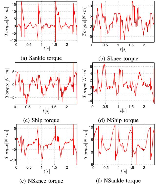
Fig. 15: Torque inputs of each motor
