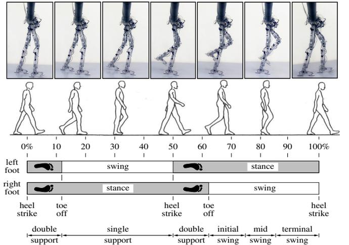
Fig. 1: Walking tiles of the multi-contact locomotion of both ATRIAS and AMBER2 (top two figures, respectively) are compared with the diagram of a typical human gait cycle.
