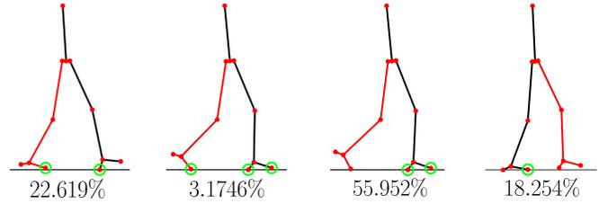
Fig. 2: Domain breakdown of one step of one subject. The numbers below each tile indicate the percentage of time spent in that domain. The green circle indicates that particular point of the foot (toe or heel) is in contact with ground. The red lines indicate the “non-stance” leg and the black lines represent the “stance” leg.
