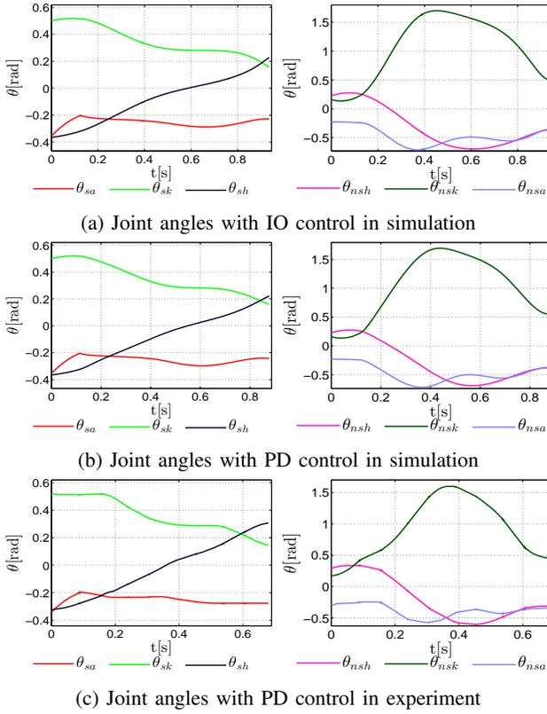
Fig. 13: Comparison of actual joint angles between simulation and experimental results logged during AMBER2 walking.
