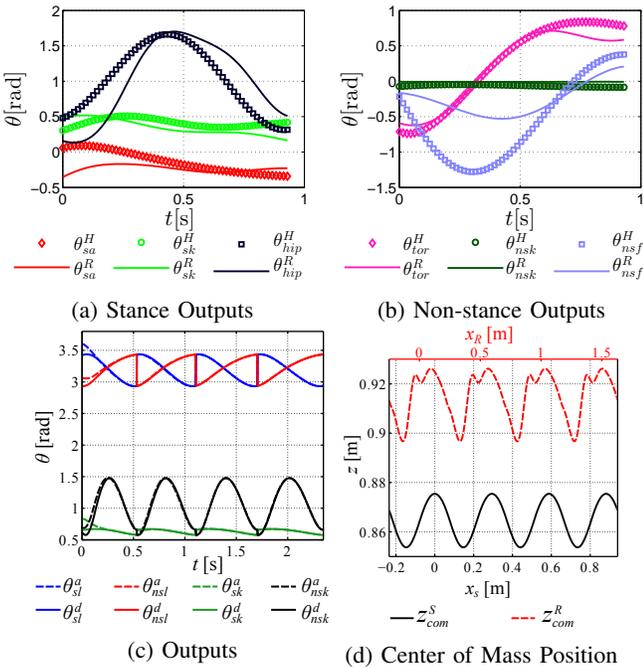
Fig. 11: Simulation results: (a) and (b) Comparisons between the human locomotion outputs and the robot outputs of AMBER2; (c) Desired versus actual outputs starting from a perturbed point of ATRIAS; (d) A comparison of the center of mass trajectory between the ideal SLIP gait and the full-order robotic model.
