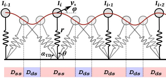
Fig. 5: The Spring Loaded Inverted Pendulum Walking Gait.
