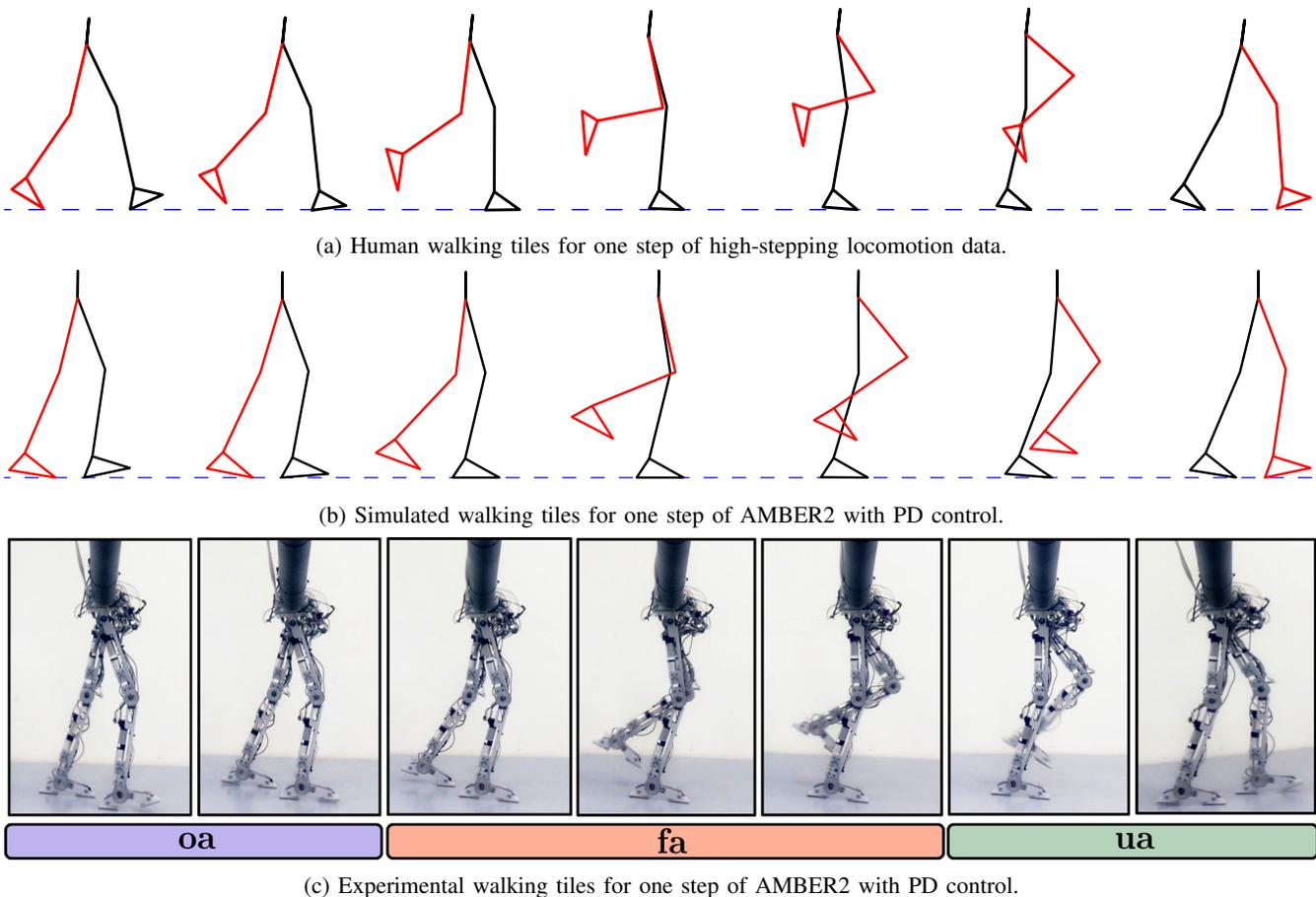
Fig. 12: Comparison of walking tiles between the actual human walking, simulated walking and experimental walking.
