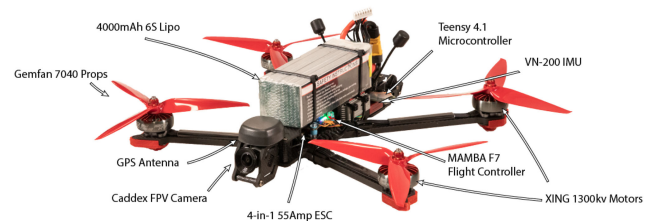
Fig. 6. The 7" racing drone used for experiments.
