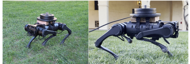
Fig. 1. The 12 kg A1 robot carrying 10 kg of payload with our method, tested for trotting in place and walking forward.
