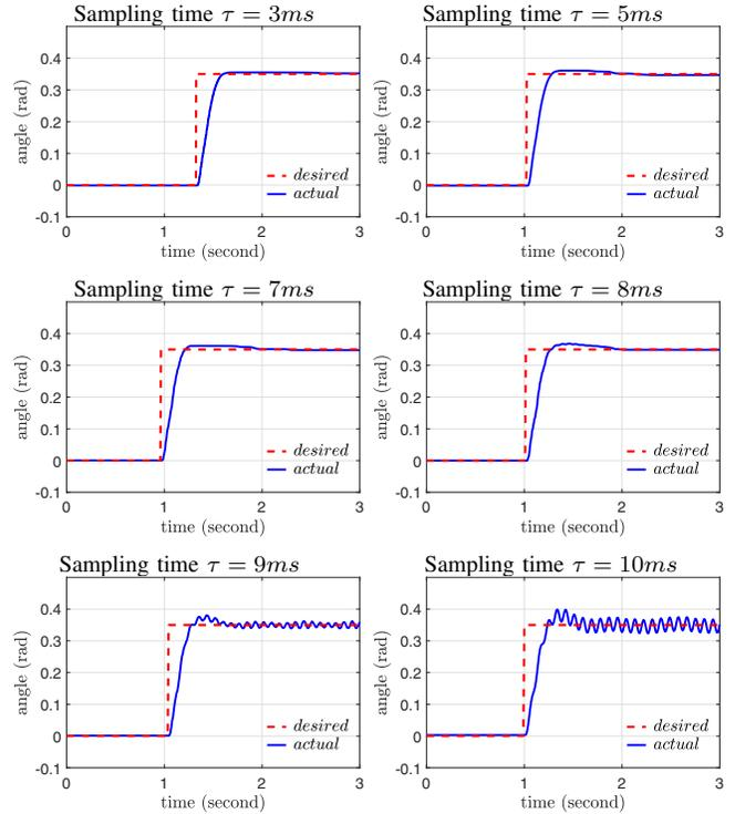
Fig. 2. Angle regulation to the desired set point of 0.35 rad for different values of the sampling time,  $\tau$ , ranging from 3ms to 10ms.
