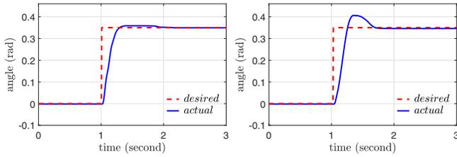
Fig. 3. Angle regulation to the desired set point of 0.35 rad when using an incorrect value for  $b$ . Left figures:  $b = 1.8$ , right figures:  $b = 4$ .
