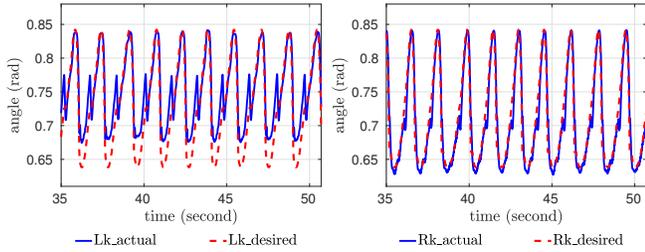
Fig. 4. Tracking performance on left (PD control) and right (data-driven control) for the knee joint while walking.
