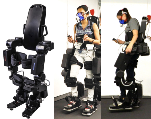
Fig. 1: Atalante Exoskeleton with and without the user. The user is wearing a mask to measure metabolic output.
